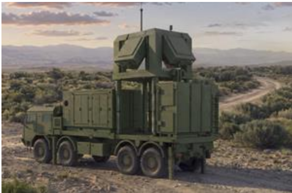
Image: Leonardo DRS' C-Band Extended Multi-Mission Hemispheric Radar, or cxMHR
